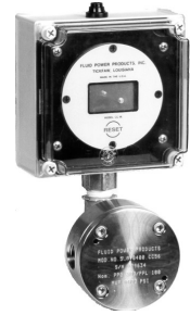
With CC56 register in NEMA 4X (= water & dust proof) enclosure
